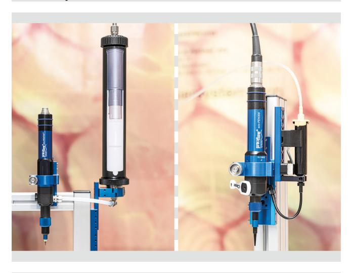
The eco-PEN is a purely volumetric dispensing system designed for applying the smallest quantities of single-component fluids. Thanks to the proven endless piston principle, it delivers fluids from watery to pasty with precision. Regardless of viscosity fluctuations, the result is a clean and process-reliable dispense.
